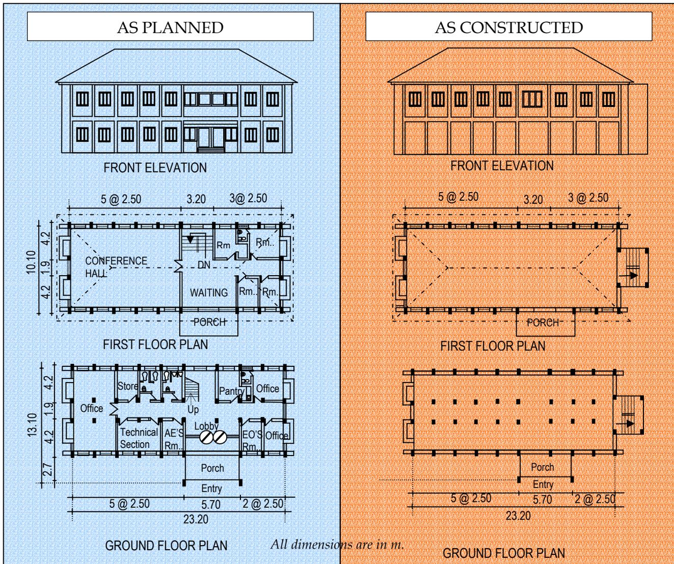
**Figure 16:** Typical plan and elevation of Panchayat buildings in the region. The 23.2 m by 13.1 m building in the plan was originally designed with office spaces on the ground floor, which was altered when built. Also, the stair case block was relocated at the end of the building.
