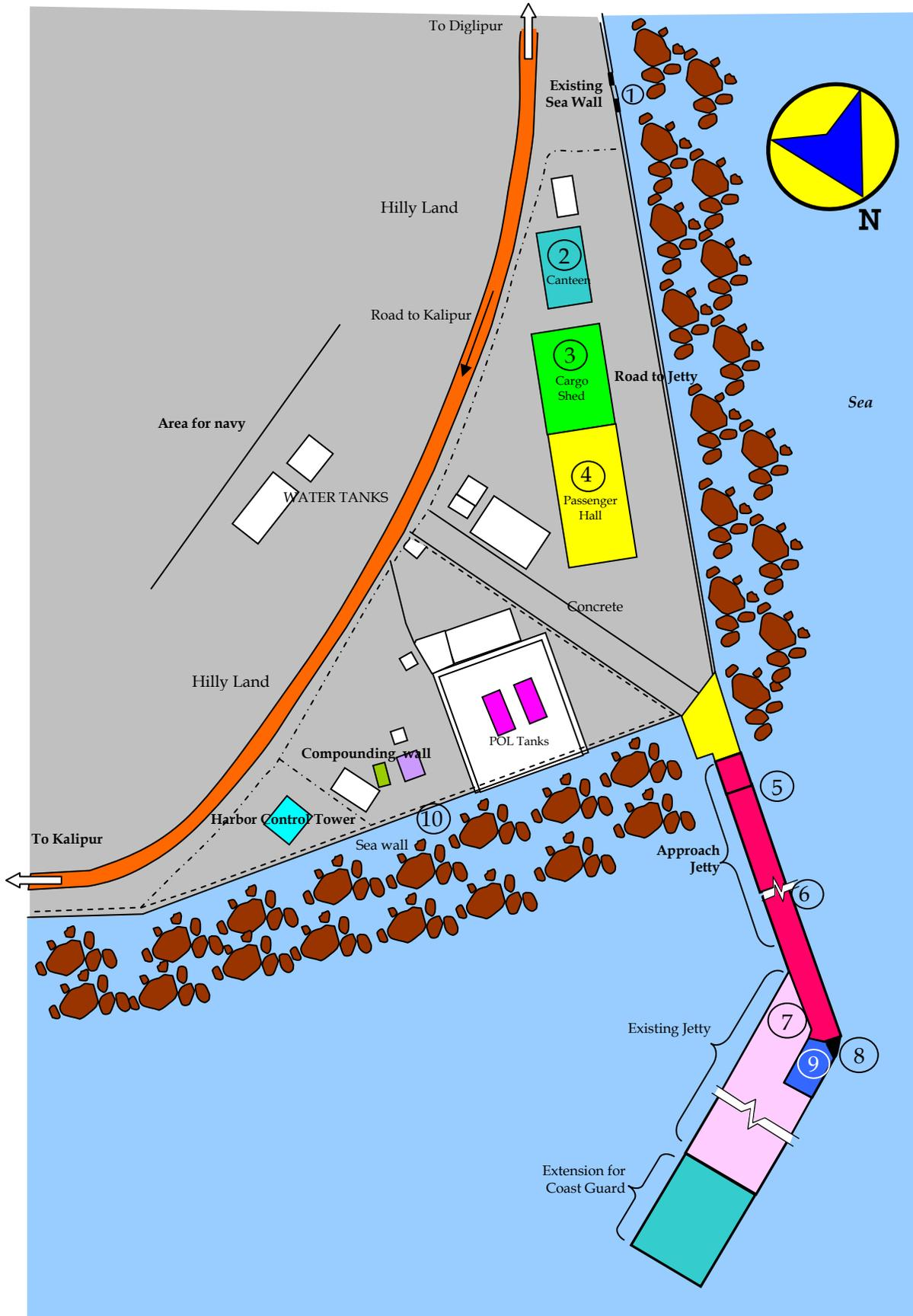
Figure 25: Map showing various structures and their arrangement at the Diglipur harbour.
