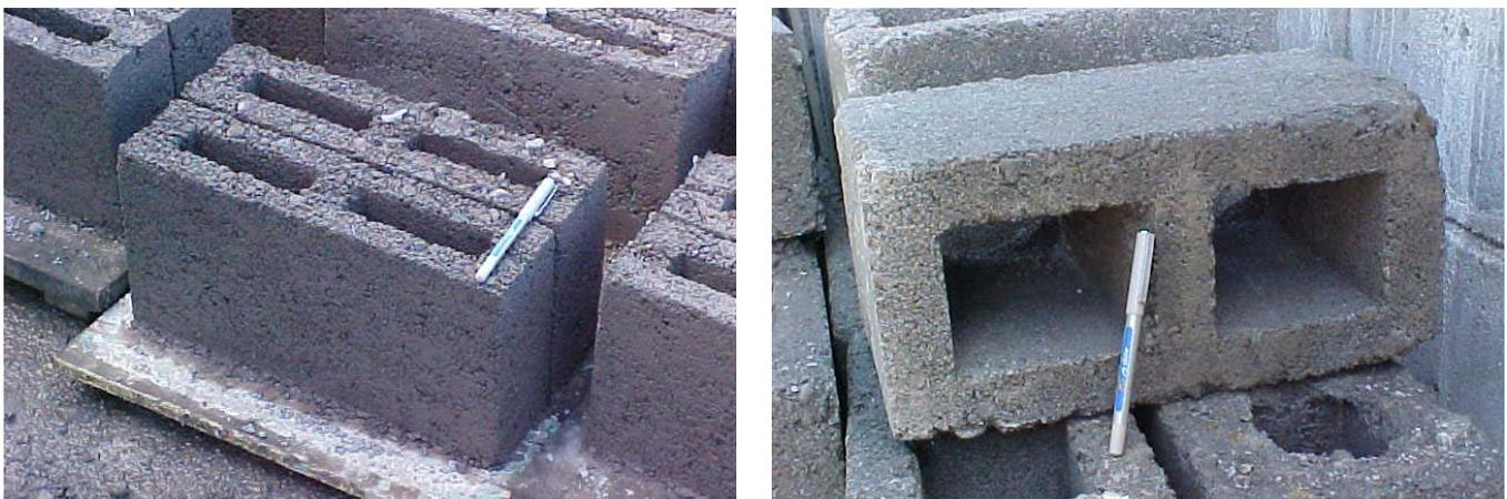
**Figure 11:** Hollow concrete blocks used for masonry wall are characterized with a very low compressive strength due to poor compaction, curing, etc.
